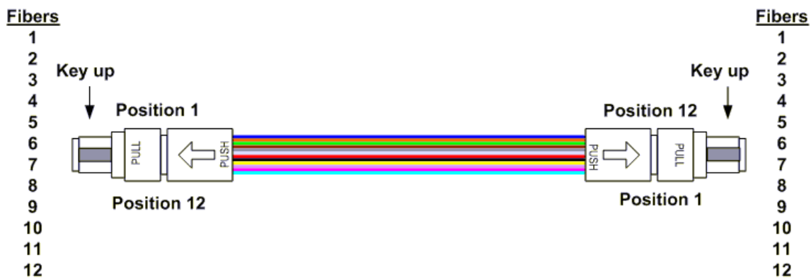
Figure 8 - Type-B array patch cord (key-up to key-up)
