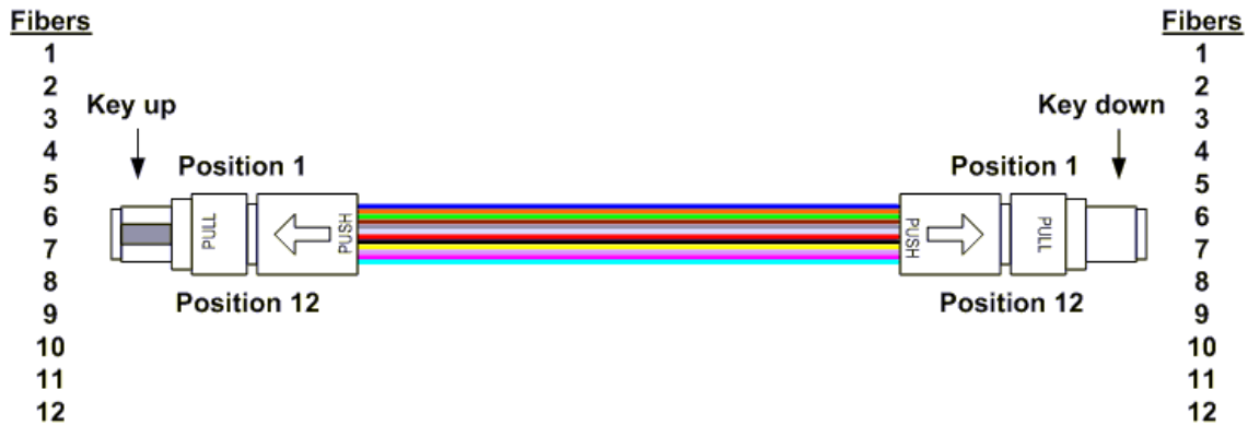
Figure 7 - Type-A array patch cord (key-up to key-down)
